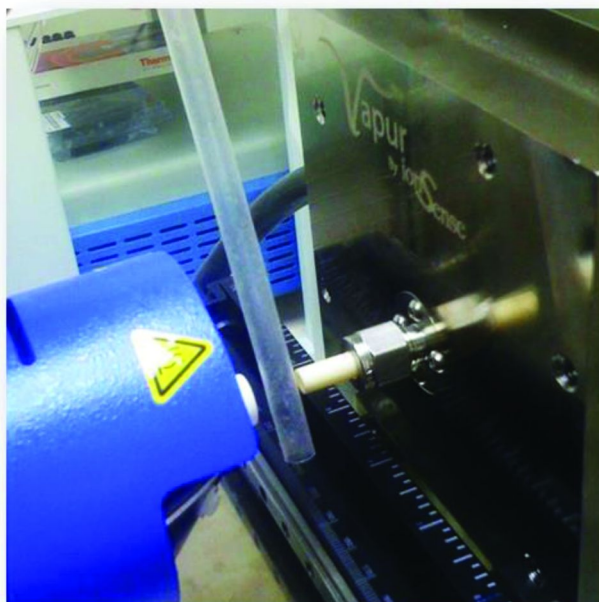
Figure 1. The DART-SVP ion source directly interfaced to the Velos Pro linear ion trap mass spectrometer. Direct phthalate screening from the surface of a plastic straw.
